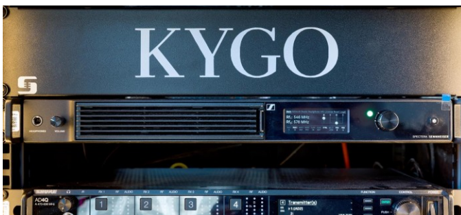
The Spectera Base Station at the monitoring console was operated with two RF wideband channels with centre frequencies of 546 and 578 MHz
